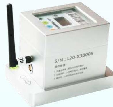
L20-X爆破测振仪
